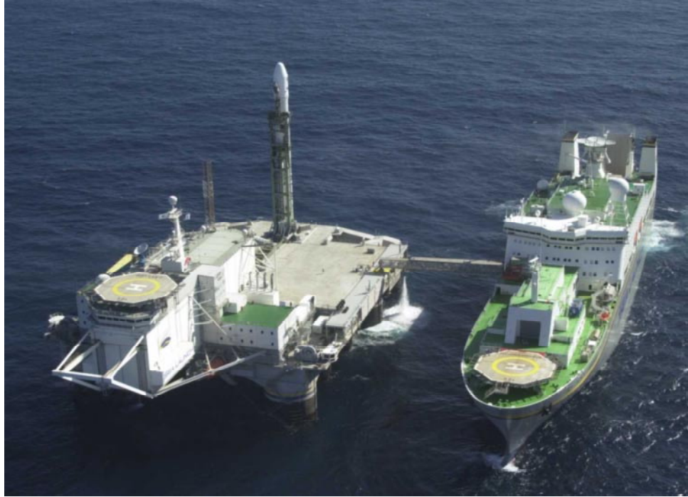
Figure 8-23. Assembly and Command Ship and Launch Platform Connected by Link Bridge
