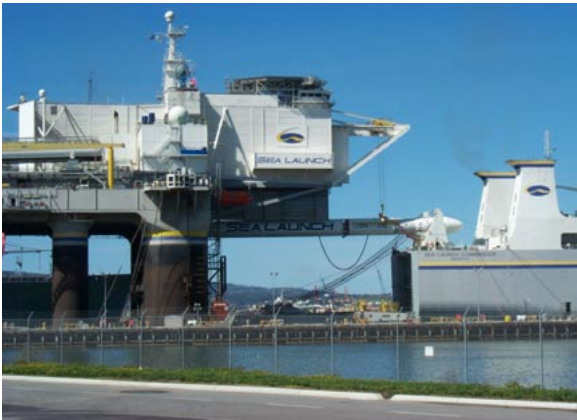
Figure 9-8. Launch Vehicle Transfer From Assembly and Command Ship to Launch Platform in the Home Port
